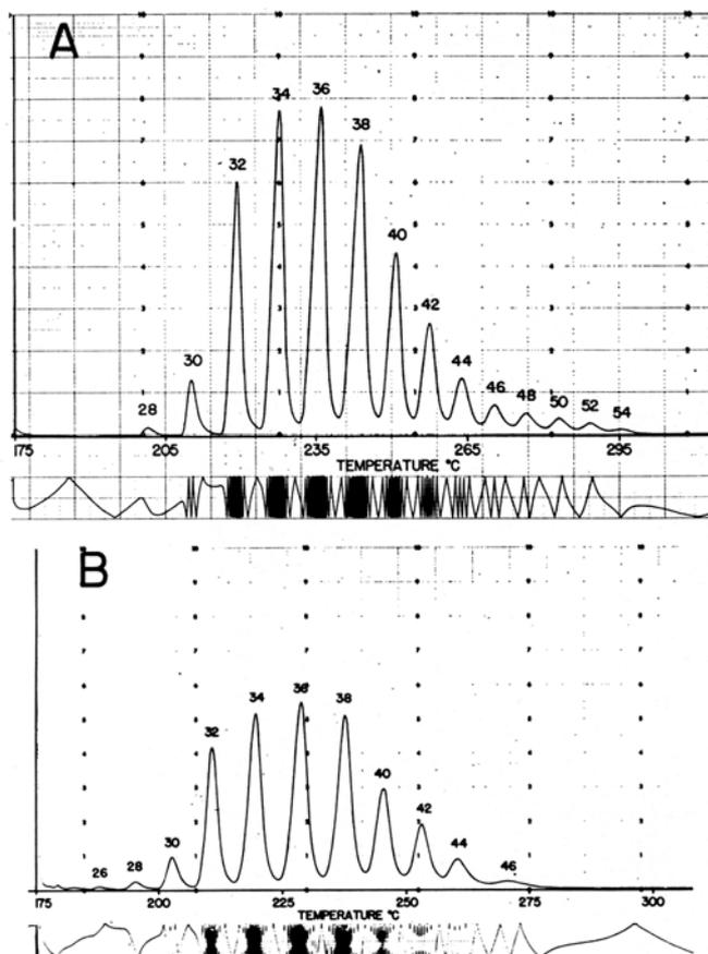
FIG. 3. Gas chromatographic separation of coconut oil on SE-30 (A) and QF-1 (B) liquid phases. Carbon number assignments and SE-30 column conditions as in Figure 1. QF-1 column: 1% QF-1 on Gas-Chrom P (100-120 mesh); 18 in.  $\times$   $\frac{1}{8}$  in. O.D.; nitrogen flow rate 100 ml/min. Other conditions as indicated in the figure. Instrumentation as in Figure 1.
