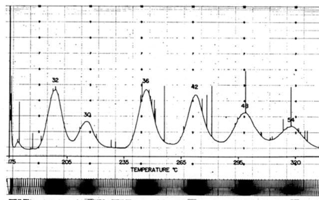
FIG. 4. Gas chromatographic separation of simple triglycerides on a low efficiency column: dotriacontane (32), tridecanoic (30), trilaurin (36), trimyristin (42), tripalmitin (48) and tristearin (54). Conditions: 3% SE-30 on Chromosorb W (60-80 mesh); 6 in.  $\times$   $\frac{1}{8}$  in. O.D. column; nitrogen flow rate 200 ml/min.; other conditions as given in the figure. Instrumentation as in Figure 1.
