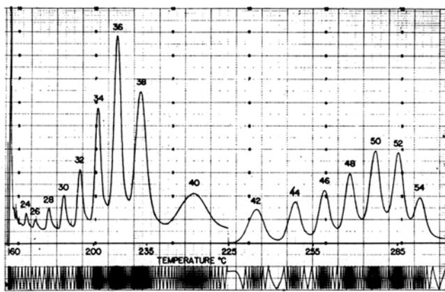
FIG. 5. Effect of changes in temperature programming upon the separation of butterfat triglycerides. Chromatography conditions as in Figure 1. After 18 minutes of programming the lid of the oven was momentarily opened.
