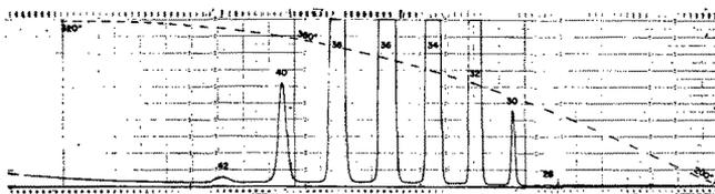
FIG. 6. GLC separation of coconut oil triglycerides in a powerstat controlled oven. Carbon number assignments as in Figure 3. Conditions: stripped 5% SE-30 on Chromosorb W (60-80 mesh); 2 ft.  $\times$   $\frac{1}{8}$  in. O.D. column; nitrogen flow rate 200 ml/min.; other conditions as given in the figure. Instrument: Aerograph Hy-Fi Model 600-C with L & N Speedomax H 1 mv recorder.
