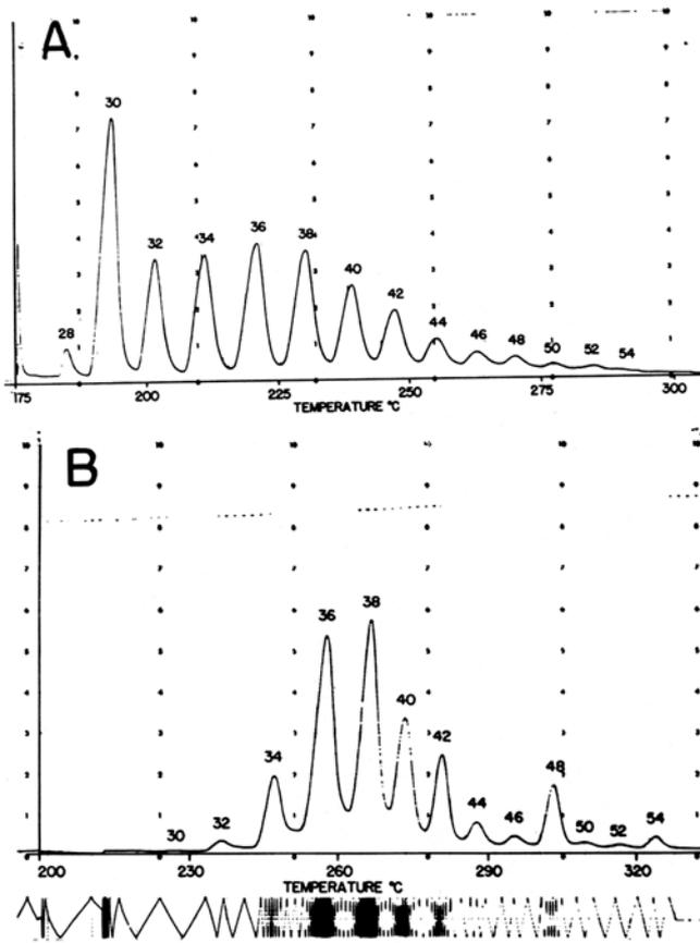
FIG. 8. Gas chromatographic estimation of triglyceride recovery of unknowns by means of internal standards. Chromatography conditions as in Figure 1: (A) coconut oil plus 25% tridecanoic acid on stripped 5% SE-30 column; (B) butter oil distillate plus 5% tripalmitin on stripped 2.25% SE-30 column.
