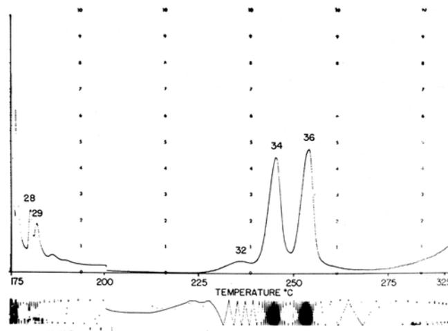
FIG. 11. Gas chromatographic separation of corn oil diglycerides. Carbon number assignments based on fatty acid composition. Chromatography conditions as in Figure 1.
